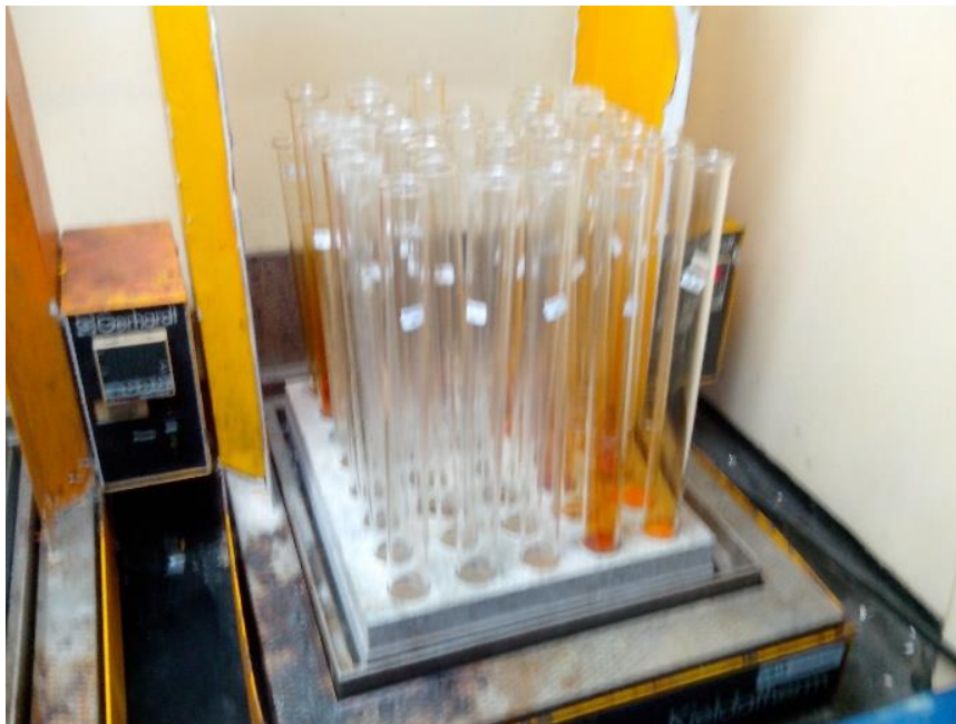
Figure 4. Acid digestion of samples
