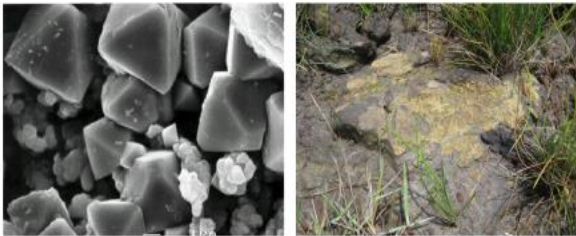
Figure 9. Oxidation of pyrite (left) results in the formation of jarosite (right)
