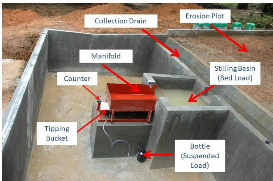
Fig. 1: Soil and runoff loss collection mechanism layout
