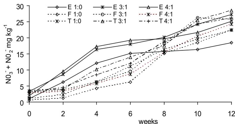
Fig. 4. Changes in  $NO_3^-$ -N and  $NO_2^-$ -N of the composting blends of oil palm wastes (E=EFB, F=frond and T=trunk) and sewage sludges at different ratios (1:0, 3:1 and 4:1) during 12 weeks of composting.
