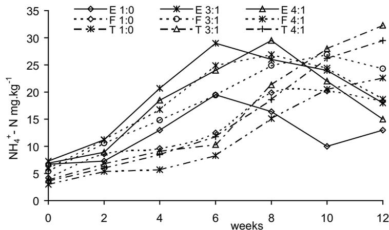
Fig. 3. Changes in NH<sub>4</sub><sup>+</sup> - N concentration of the composting blends of oil palm wastes (E=EFB, F=frond and T=trunk) and sewage sludges at different ratios (1:0, 3:1 and 4:1) during 12 weeks of composting.
