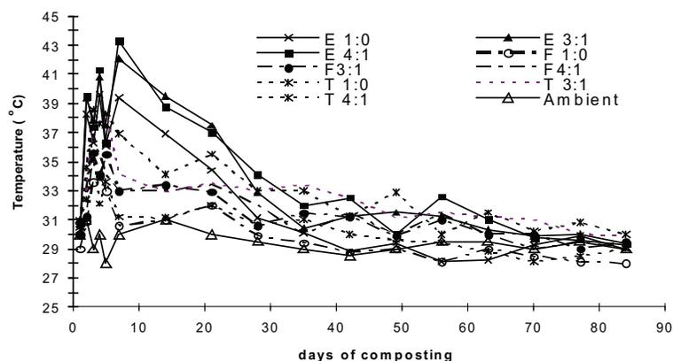
Fig. 1. Changes in temperature of the composting blends of oil palm wastes ( $E$ =EFB,  $F$ =frond and  $T$ =trunk) and sewage sludge at different ratios (1:0, 3:1 and 4:1) during 12 weeks of composting.
